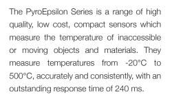
PyroEpsilon sensors transmit the target temperature as a 4-20 mA output and offer a simple solution for most non-contact temperature measurement applications.
