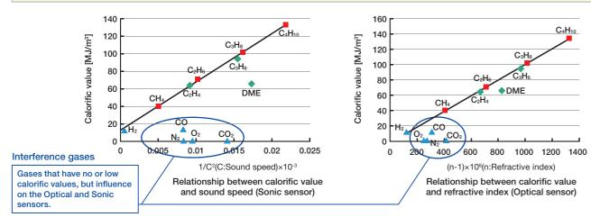
"Opt-Sonic calculation" using measuring results of the Optical sensor and Sonic sensor can minimize the interference effects caused by interference gases, and realize a high-accuracy measurement.
