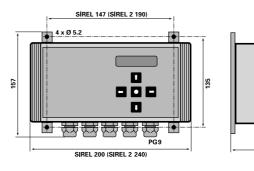
SIREL control unit for 1-angle measurement
